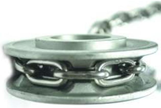
For chain blocks to be used up to an angle of 45 degrees, it's critical that the hand chain leaves and enters the hand wheel without twisting, snagging or jamming. Thanks to our specially designed deep-profile chain block hand wheel this is achievable as it helps to seat the chain no matter what angle or direction of pull.
