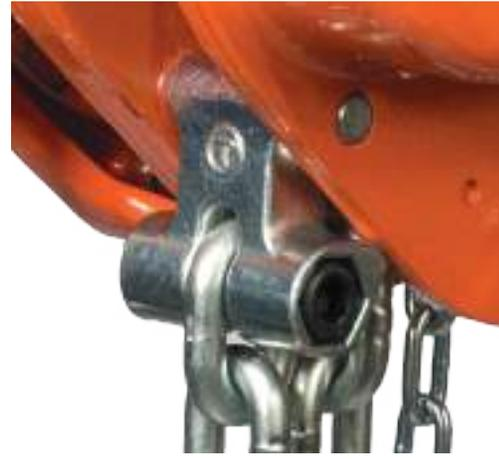
Our chain end anchors will hold a load of at least 2.5 times the rated capacity when supporting the full load without restraint from other components e.g. brake or gearing. This prevents accidents, by acting as a stop when the lift length of the load chain is exceeded when lowered. The image shows our special strong and contoured design used on our PROCB and SS20 ranges.
