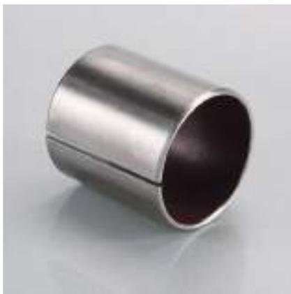
We have incorporated DU® self-lubricating metal polymer bearings into our multi chain fall load sheaves. Their high wear resistance and extremely low friction properties makes them ideally suited to hoists used subsea.
