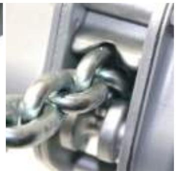
The fluted chain stripper is specifically designed to guide the load chain safely onto or off the load sheave. The critical configuration of, and distance between, the chain stripper and the roller guide ensures alignment of the chain so it cannot snag or jam. This allows the safe use of the SS19/PROLH when used in any orientation.
