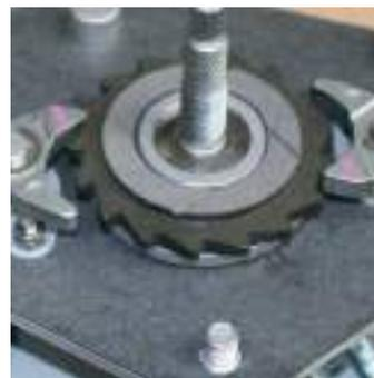
The SS19 has bonded marine friction discs developed and designed for subsea use creating a highly efficient, reliable braking surface for use in the most extreme conditions.
