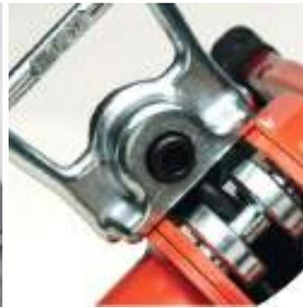
User friendly heavy duty end stops on our PROLH (and as an option on our TR7) make it easy for the operator to position the chain while "freewheeling". Most importantly this "end stop" will hold a load of at least 2.5 times the rated capacity when supporting the full load without restraint from other components e.g. brake or gearing.
